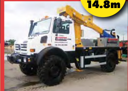
VERSALIFT VST240i PLATFORM Mercedes Unimog U5000 (with Category C Insulation)
