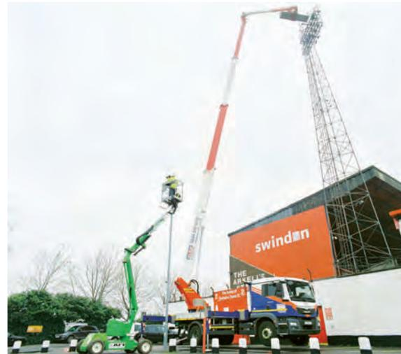
The green Niftylift HR12 works beside the 45m truck-mounted boom at Swindon's ground
