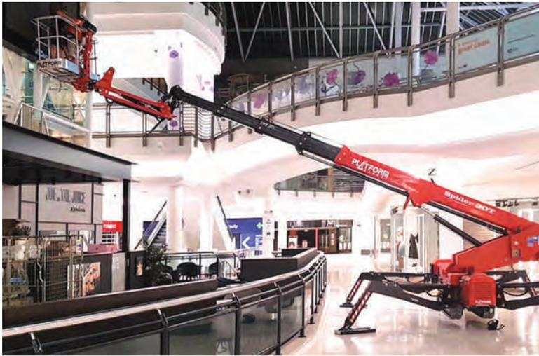
Italian manufacturer Platform Basket's Spider 30T hybrid model has a 30.3m maximum working height
