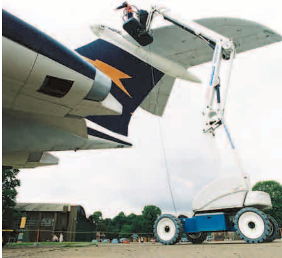
Rapid Platforms' Niftylift HR21 was able to reach the VC10's tailplane
