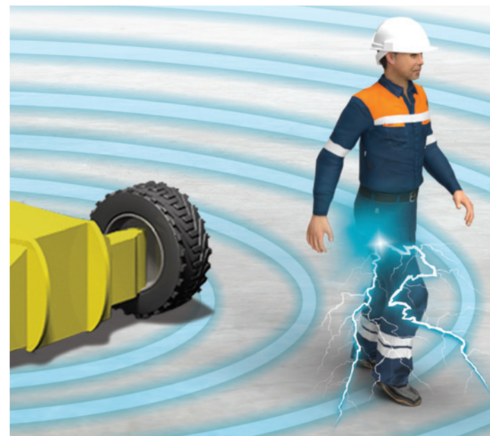
Figure 2 Image showing scenario where person could be at risk of electrocution or electric shock.
